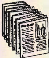
STEP 3—COLLATING (GATHERING) THE SIGNATURES IN THE CORRECT ORDER
