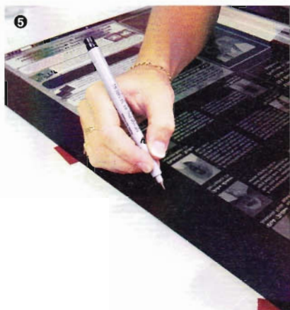
Cover any nonimage marks with opaque.
