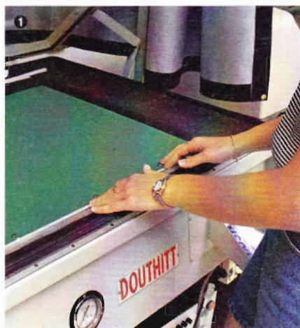
1 Insert the plate into the vacuum frame.
