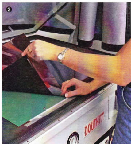
2 Place the flat on top of the plate in the vacuum frame.
