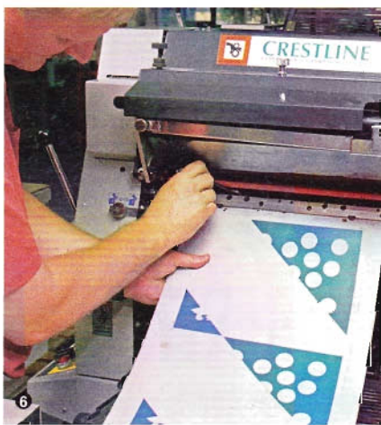
Mount the plate on the press.
