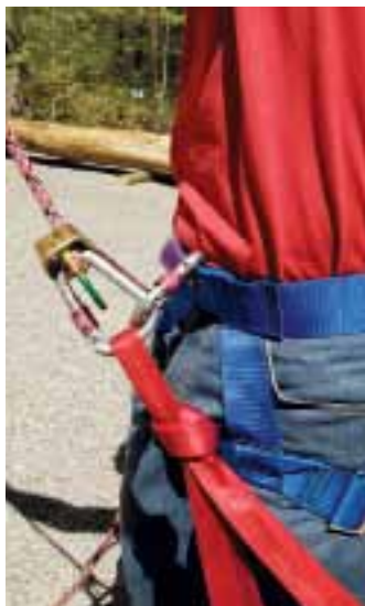
Bottom belay system setup
