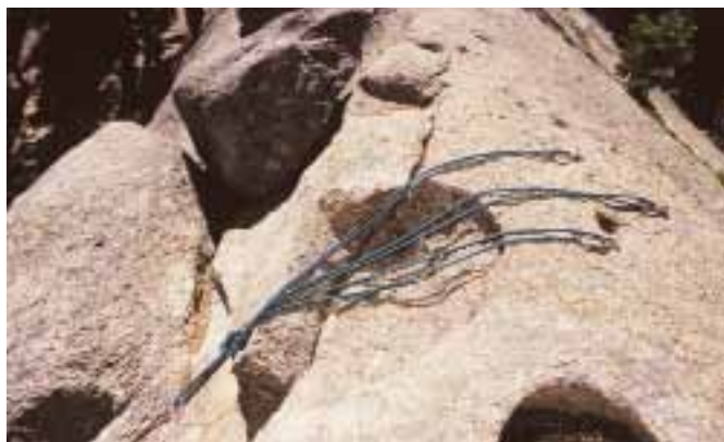
A cordelette anchor system divides the force of a load among several anchor points.
