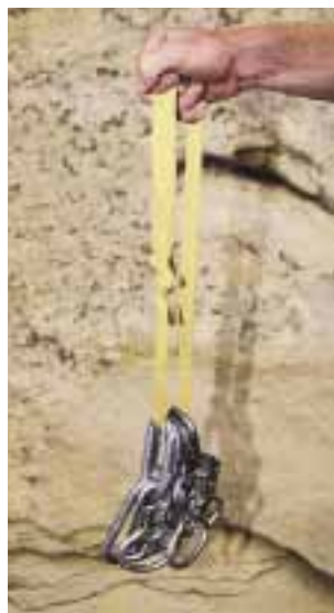
Gear slings or short lengths of webbing can be used to help organize climbing gear.
