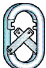
Always use nonlocking carabiners in pairs, with the gates of the carabiners reversed.
