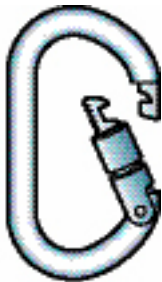
The locking carabiner protect against accidental opening.
