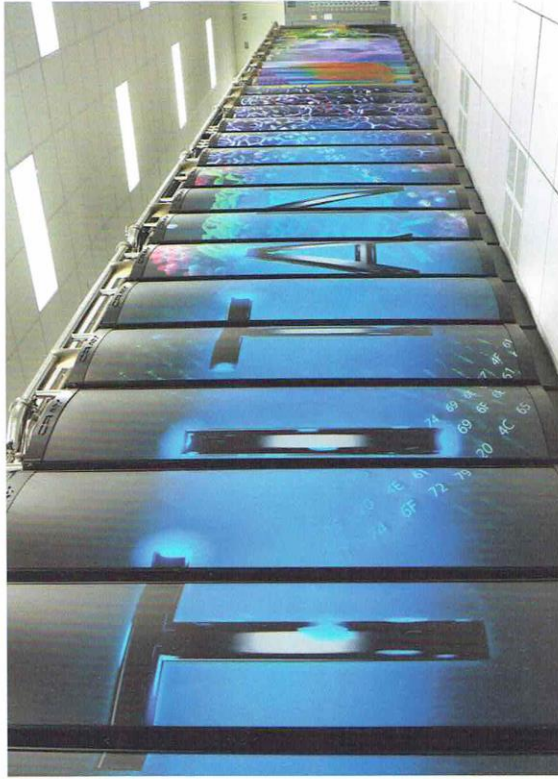
The supercomputer is the fastest type of computer made. This is Titan, one of the world's largest supercomputers.
