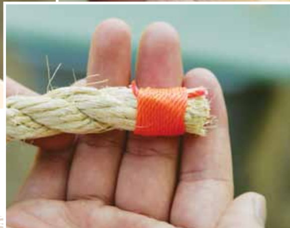
Steps in whipping the end of a rope
