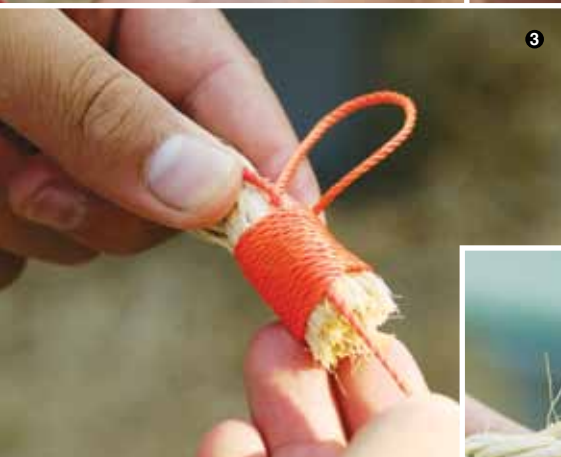
Steps in whipping the end of a rope
