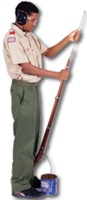
Clean the breech and barrel of your percussion model by using a flush-out nipple.
