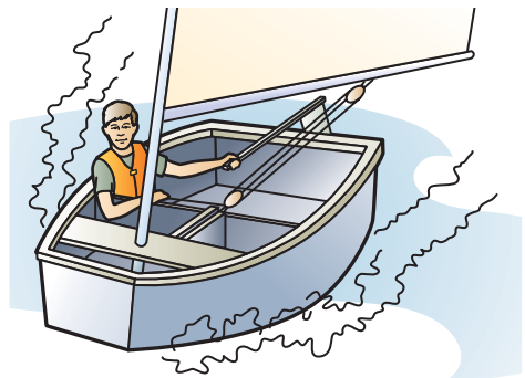
The freestanding mast of an Optimist pram needs no standing rigging.
