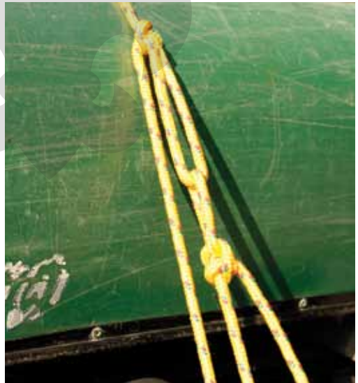
Secure the kayak to the racks using cam straps, bungee cords, or lines using a trucker's hitch. The lines should be tight and secure, but be careful: It is possible to tighten hard enough to damage the hull.
