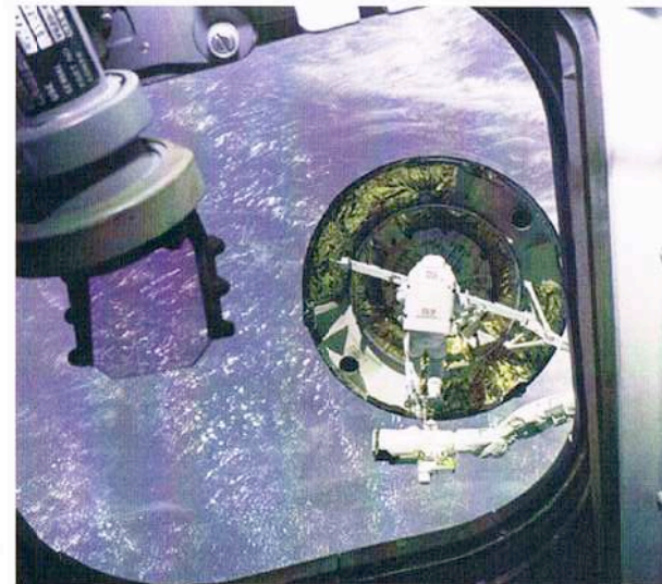
This photo, taken from the shuttle's aft (rear) flight deck windows, shows an astronaut from the space shuttle Endeavour trying to capture the Intelsat VI communications satellite.
