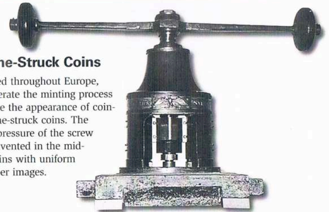
A screw press, used at the Paris Mint in the 1780s
