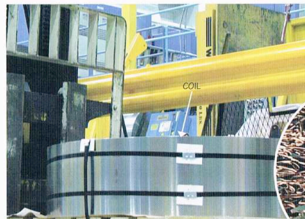
Each coil is about 12 inches wide and weighs around 6,000 pounds.
