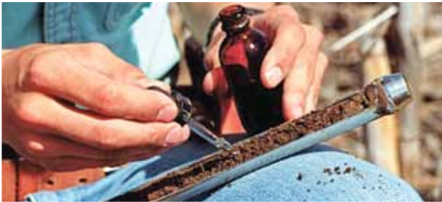
A soils expert tests a soil core to determine its pH—how acidic or alkaline it is.
