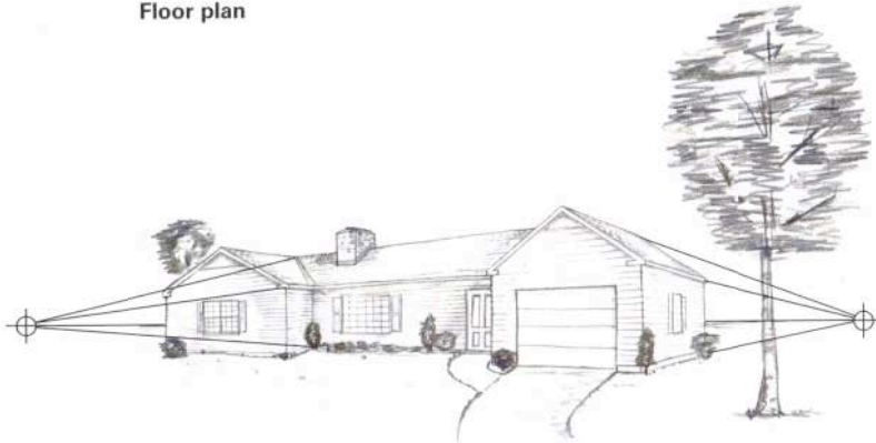
If you draw lines from the "horizontal" lines of the house pictured, they meet at the vanishing points .
