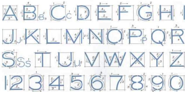
Mechanical and electrical lettering
