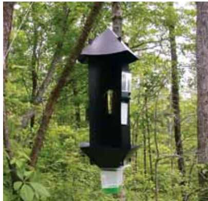
Scientists use this flight intercept trap to help them study adult red oak borers.
