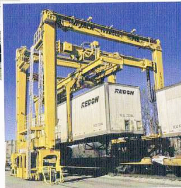
For containerized cargo, flatcars are frequently loaded and unloaded by an intermodal crane, which straddles the train.
