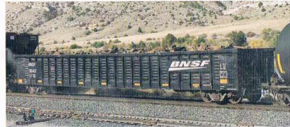
Mill gondolas provide the maximum open carrying capacity for exposed loads. For protected loads such as steel coils, gondolas are equipped with removable covers. Side-dump gondolas can unload by tilting to either side; coal-carrying gondolas unload by turning upside down.
