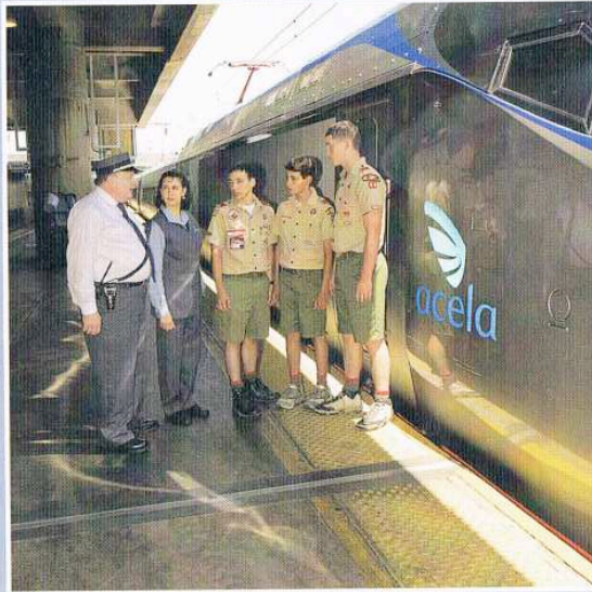
The Acela Express is called a trainset because the cars—electric locomotives at each end and six coaches in between—operate as one unit.
