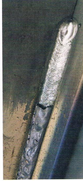
Slag peeling off shielded metal arc welding workpiece
